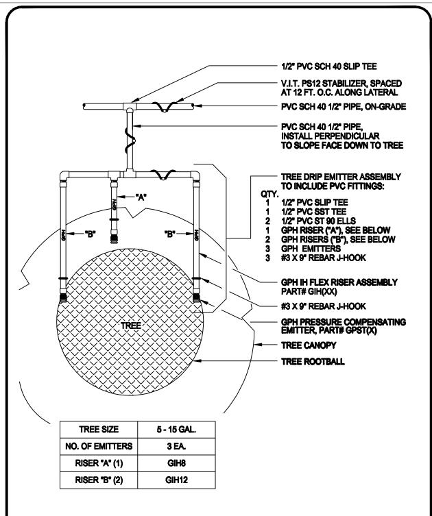
EMITTERS SHALL BE INSTALLED AT EDGE OF TREE ROOTBALL AS SHOWN. ALL IRRIGATION EQUIPMENT SHALL BE INSTALLED PRIOR TO TREE LAYOUT AND PLANTING.
